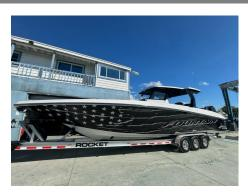
LOA - 38' 4" Beam - 10' 6" Weight (Approx.) - 15,600 lbs. Fuel Capacity - 425 gal. (one tank) Water Capacity - 34 gal. Bridge Clearance - 112" Draft (Max Drives Down) - 31" Deadrise - 20.75° Max Horsepower - Mercury Quad 500Rs
